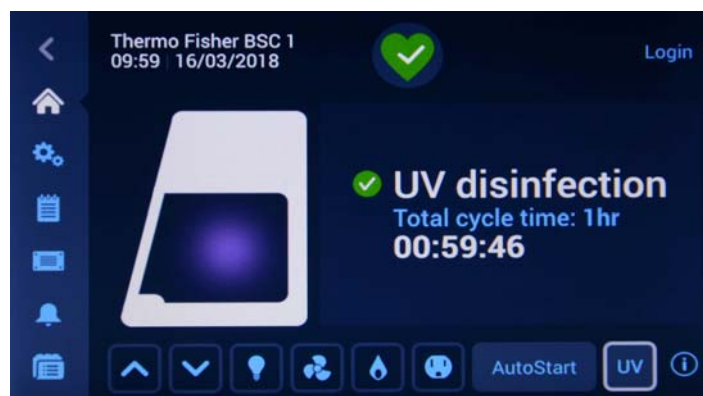
Figure 42 Main Screen: UV Disinfection Running
