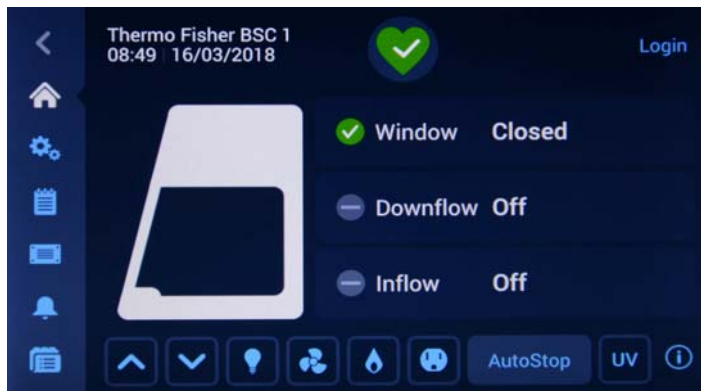
Figure 35 Main Screen - Unit in Idle State, Window Closed
