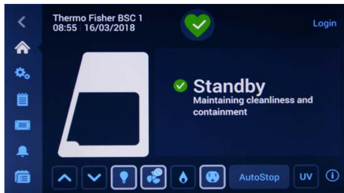
Figure 33 Main Screen - Unit in Standby
